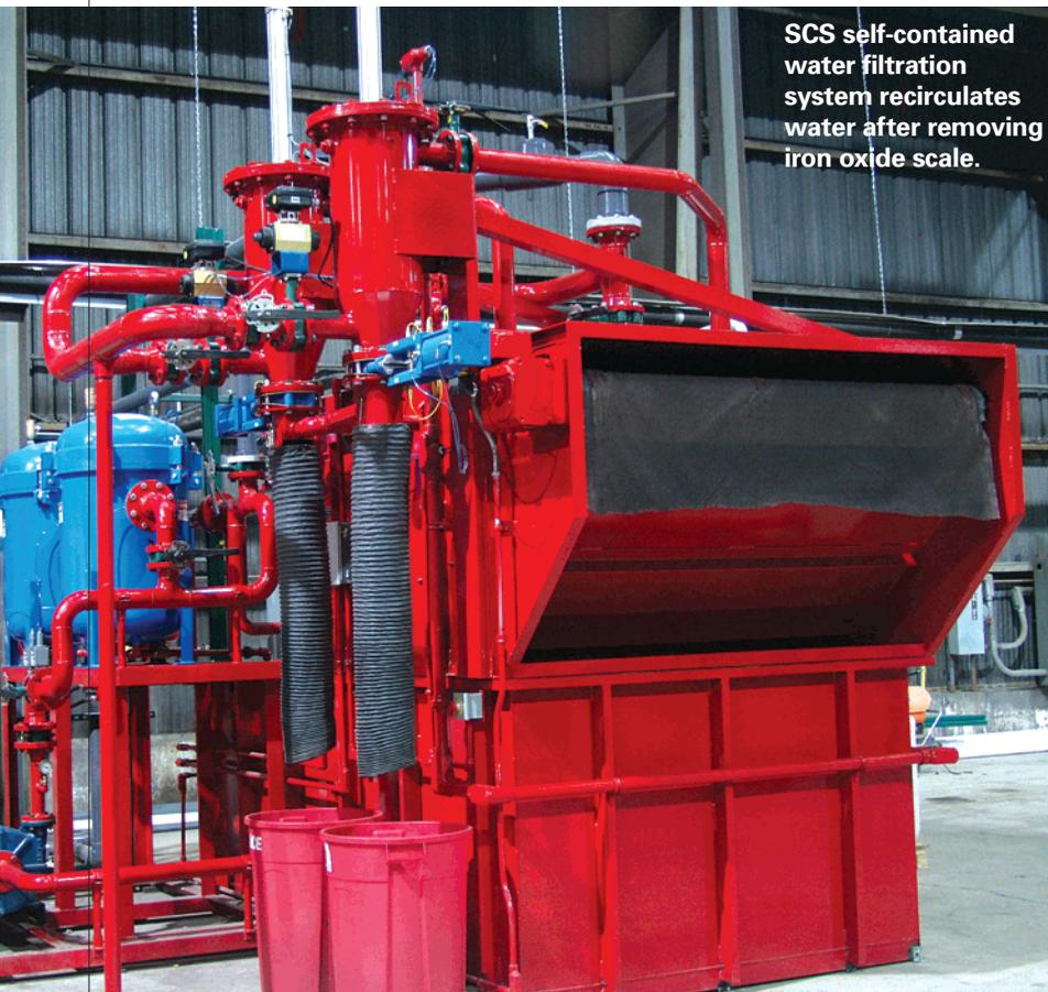
SCS self-contained water filtration system recirculates water after removing iron oxide scale.
