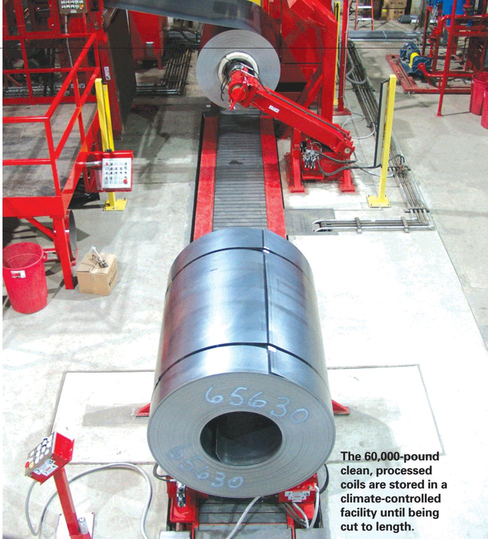
**The 60,000-pound clean, processed coils are stored in a climate-controlled facility until being cut to length.**
