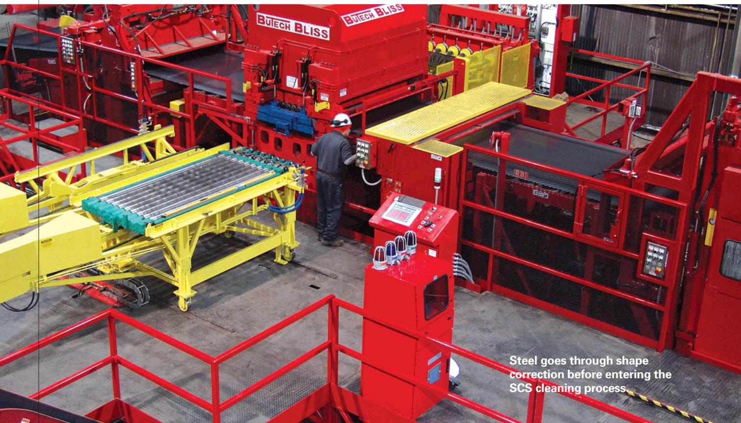
Steel goes through shape correction before entering the SCS cleaning process.
