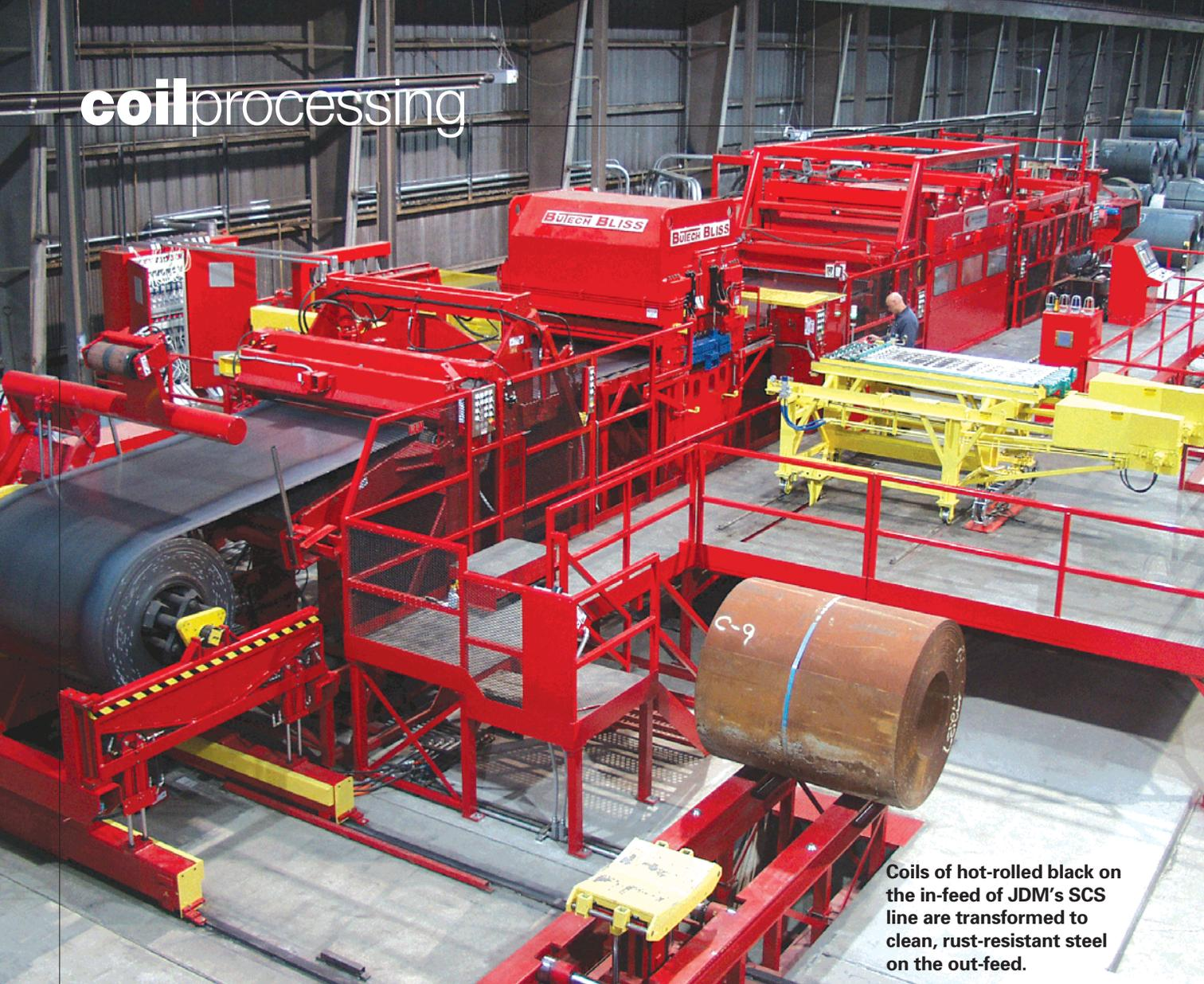
Coils of hot-rolled black on the in-feed of JDM's SCS line are transformed to clean, rust-resistant steel on the out-feed.
