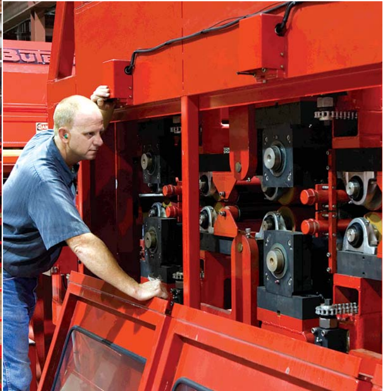
Tim Voss, lead technician at TMW, inspects the cleaning section of the SCS coil line. Three pairs of brushes are flooded with water at 180 gallons per minute, and the closed-loop system eliminates municipal sewer discharge.
