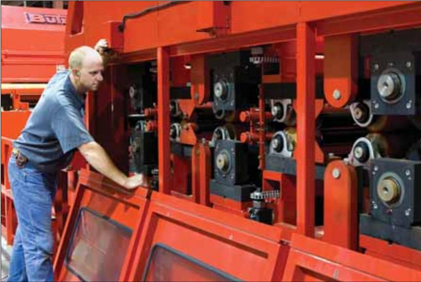
⬇ A technician examines the interior of TMW's patented SCS brush machine, which uses either an abrasive 3M Scotch-Brite pad or brushes with nylon-coated silicon carbide bristles to remove rust, dirt and scale from the steel.
