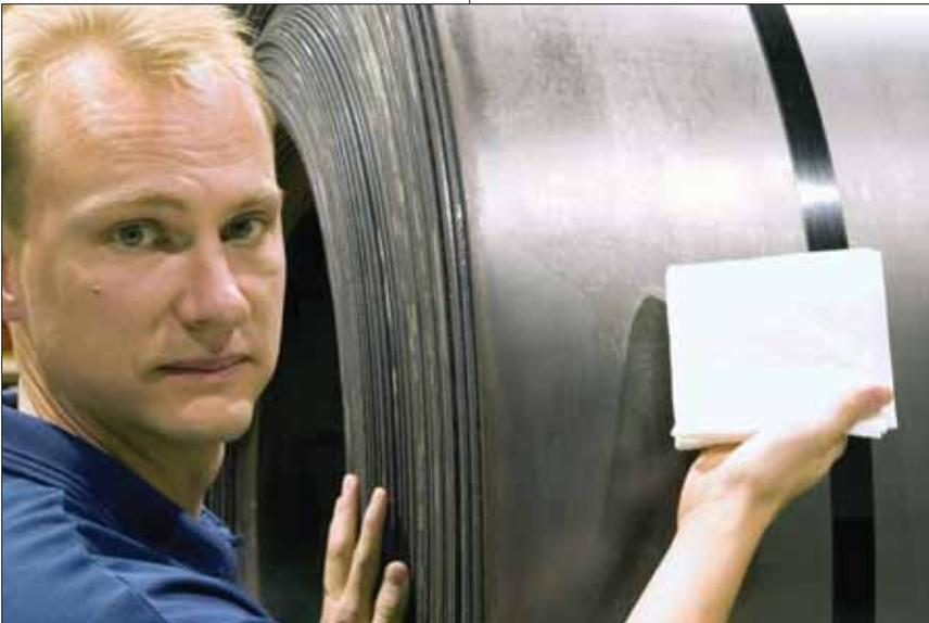
⬆ The SCS system can take a dirty, rusty commodity-grade coil and give it a napkin-clean surface ready for painting. The SCS process leaves a microscopic layer of scale on the steel, which inhibits rust, the company says.
